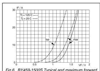
Fig.6. BY459-1500S Typical and maximum forward characteristic  $I_F = f(V_F)$ ; parameter  $T_j$
